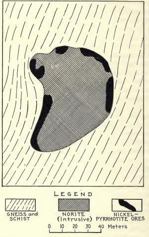
Fig. 93.—Nickel-pyrrhotite ores on the margin of an intrusive norite dome. Bamle, Norway. After Vogt, Zeit. f. prakt. Geol.; 1893, Plate VI.
